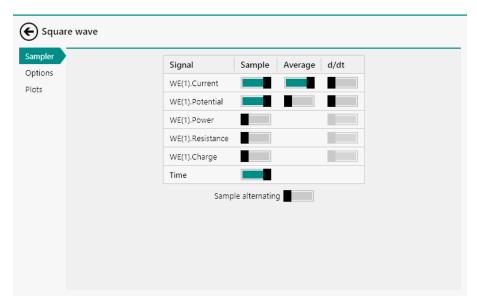
Figure 657 The sampler of the Square wave command
