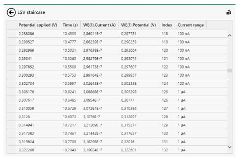
Figure 30 The active current range is now reported in the data grid
