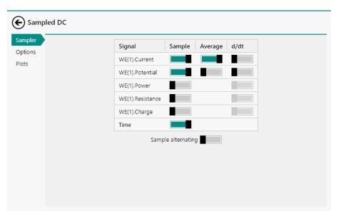
Figure 628 The sampler of the Sampled DC command
