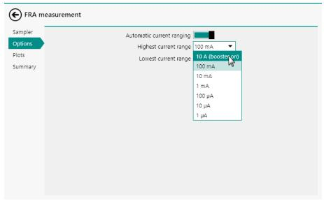
Figure 364 The current range of the Booster10A and Booster20A is available in the Automatic current ranging option
