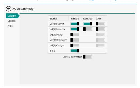
Figure 664 The sampler of the AC voltammetry command
