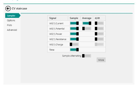
Figure 759 The sampler defines which signals are measured or calculated by the command
