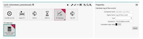
Figure 406 Using the Calculate signal when stacked onto another command
