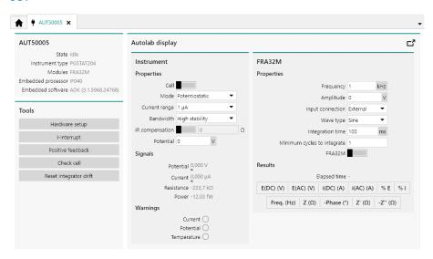
Figure 94 The single channel Autolab control panel
